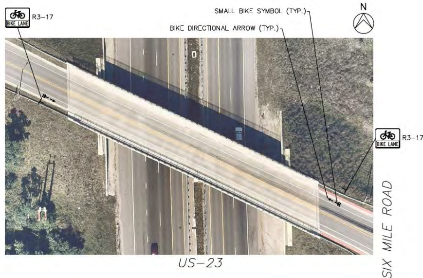
Figure 54: Proposed Bicycle Signs and Pavement Markings at Six Mile Road Crossing US-23
