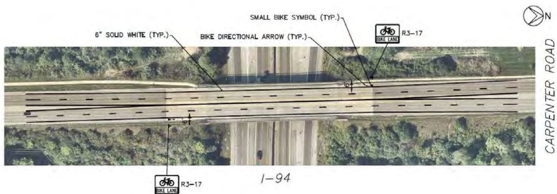
Figure 18: Proposed Bike Lanes and New Lane Geometry at Carpenter Road Crossing I-94
