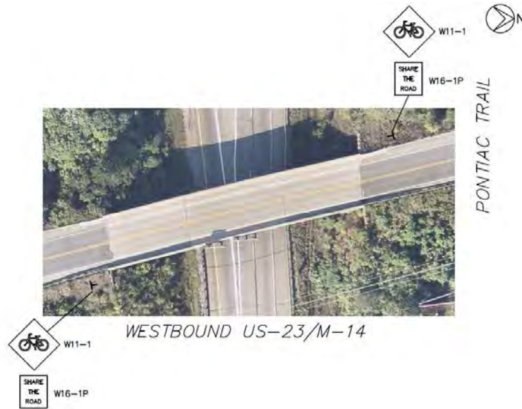
Figure 84: Proposed Bicycle Warning Signs and Plaques at Pontiac Trail Crossing Westbound US-23/M-14
